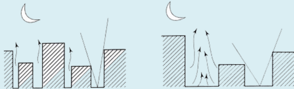
Fig D4.2: Greater the exposure of the walls and ground to sky, more the heat loss
